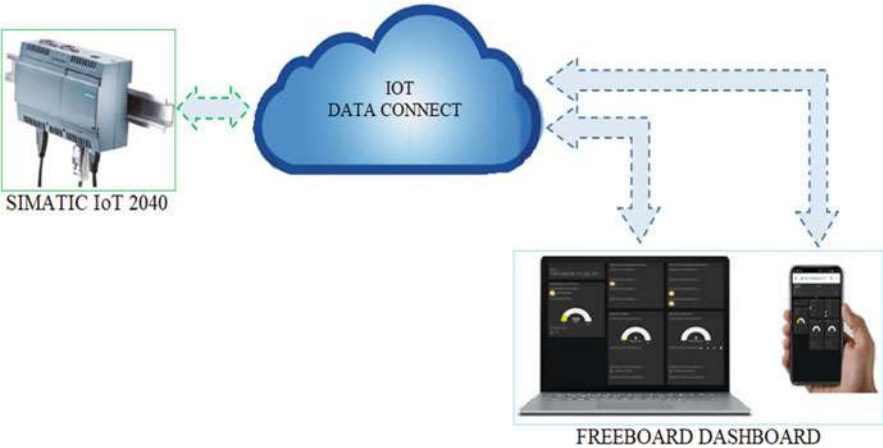
Fig. 14.7 Communication between the Simatic Iot2040 Gateway and the Freeboard Platform
