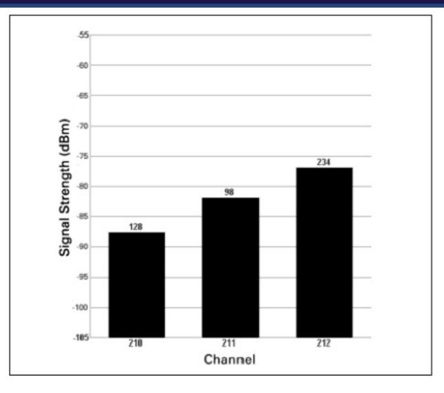
The process of identifying the interfering base station is simplified if a drive-test tool is able to provide the channel number, power level of the interfering signal and the DVCC of the interfering signal. In addition, the DVCC of the signal on channel 212 is shown on top of the bar. In this case the DVCC is 234.
