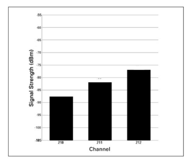
Bit errors will occur on channel 211 due to the strong signal present on channel 212. Knowing that the interfering signal is on channel 212 is useful. A channel plan can now be used to determine the source of the strong signal on channel 212. First, examine the channel table for channel set D3, of which channel 211 is a member. For this example assume that the serving sector is 5. Notice that the techniques of alternating Terminal equipments analysis for IMT 2000 Network platform
